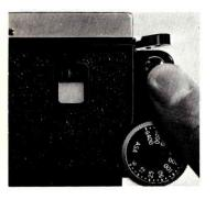
The Photomic FTN Finder is powered by two 1.3 volt mercury batteries located in the battery chamber on the bottom of the finder. To check the batteries, press the meter switch-off button and observe the needle in the window on top of the finder. If the needle swings to the center circle or beyond, the batteries are in good condition. The two mercury batteries come installed with the Photomic  $FT_N$  Finder.
