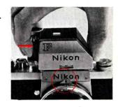
To remove the finder, depress the finder lock lever and press the finder release button located on the back of the camera. The finder will be unlocked and can be lifted out.
